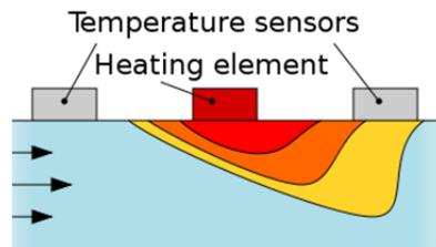
Figure 3 - Thermal Mass Flow Sensor
