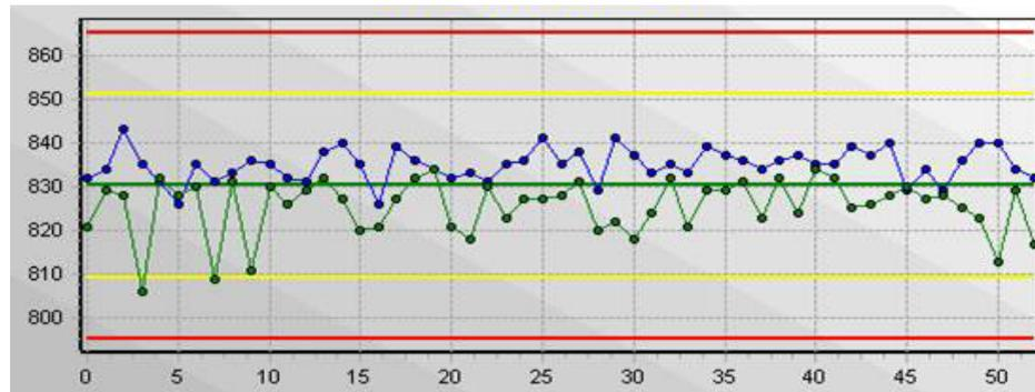
Figure 5 – SPC charts for 2 bowls, in  $\mu\text{L}$  per dispense (300 mm fab). The green line contains suspect dispense events with external variations that call for maintenance.
