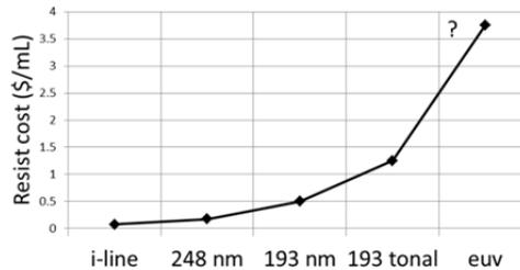
Figure 1 - Resist cost per mL as a function of light source linewidth
