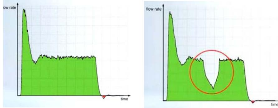
Figure 4 - Dispense profiles as measured by a MEMS sensor. The profile on right shows an air bubble. MEMS sensors are able to measure reverse flow (suck back) (red area in both profiles).
