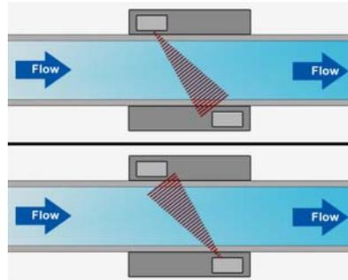
Figure 2 - Ultrasonic flow meter. Speed is inferred from the delay between the 2 signals.
