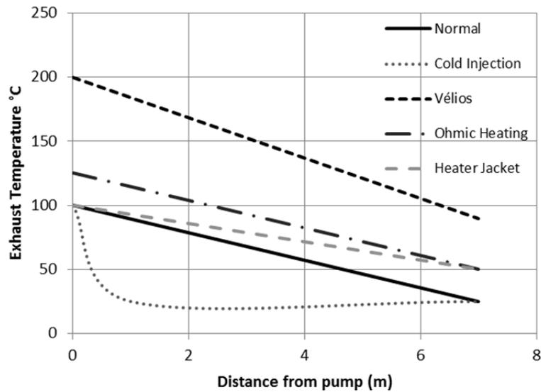
Figure 4 - Exhaust temperature profile for various dilution techniques. These examples are for normal operating conditions and an initial exhaust temperature of 100 °C. On-board heating would change the starting temperature.
