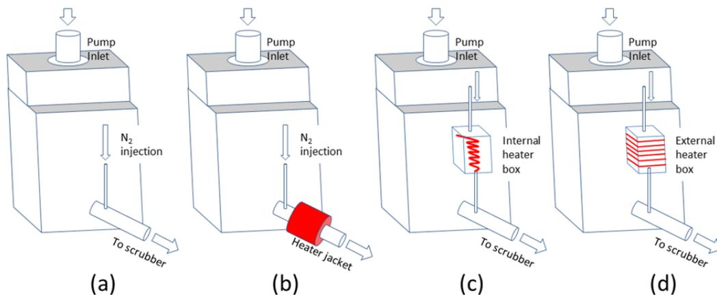
**Figure 2 - Various dilution techniques: a) Room temperature  $N_2$  injection, b) Injection with heater jacket around exhaust line, c) Hot injection with internal heated filament, d) Hot injection with external filaments.**
