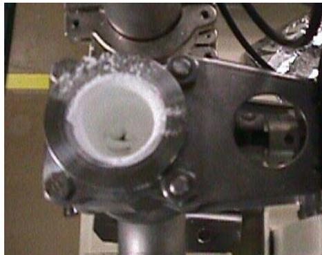
In some cases, catastrophic clogging can occur, causing gas flow to reverse and condensate matter to flow upstream into process tools, necessitating extensive cleaning and requalification.
