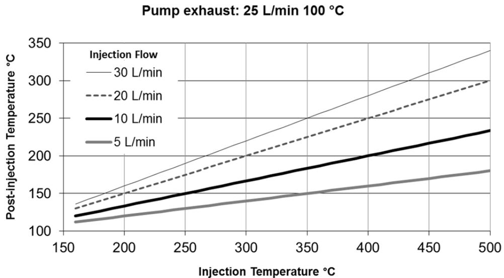
Figure 3 - Post injection temperature for various injection flows and temperature combinations when using an IR heater. In this example, the pump flow is set at 25 L/min and the initial exhaust temperature is 100 °C. Actual operating conditions may vary.
